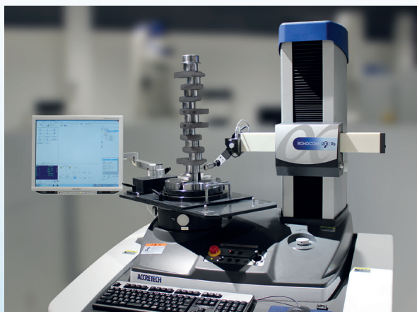
Measuring crankshaft using designated jig tool
