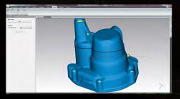
generated triangle mesh with cross-section selection
