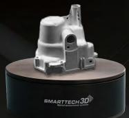
**SMARTTECH3D UNIVERSE** is a 3D scanner that combines high accuracy of measurement for reverse engineering and the possibility of scanning realistic color texture necessary for digitizing objects.
